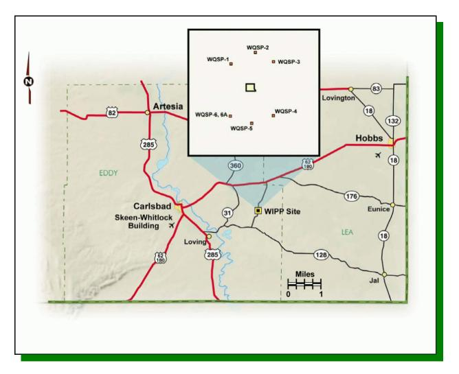
Figure 6.1 - Water Quality Sampling Program Wells (Inset represents the locations of the DMP wells in the four-square-mile area of the WIPP site [Land Withdrawal Area].)
